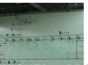
A production board is installed depicting outputs, monitoring the production status of the enterprise. A simple addition that encourages efficiency.
