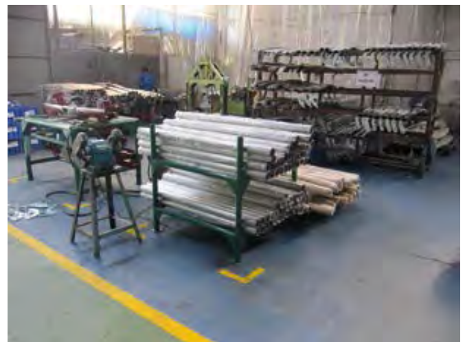
After: Clean and tidy production area with proper built-in racks to store part and materials, as well as the usage of yellow lines to divide work sections.
