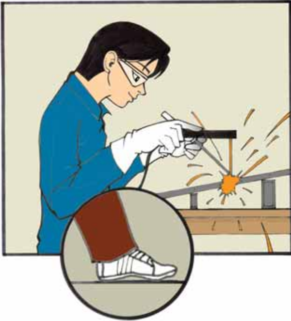
Figure 67: Use appropriate shoes, gloves and other protective devices to protect home workers.
