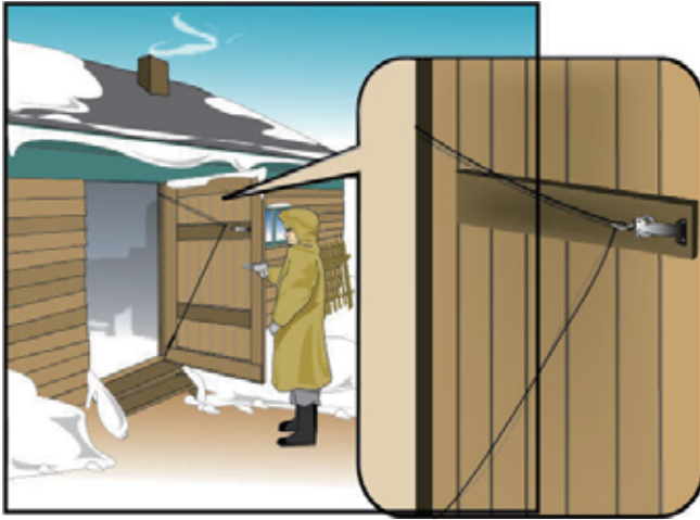
Figure 57: Simple spring device to close the door automatically after opening.
