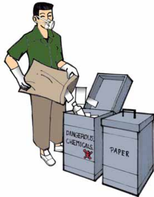
Figure 55: Collect waste bottles of dangerous chemicals in a separate container.
