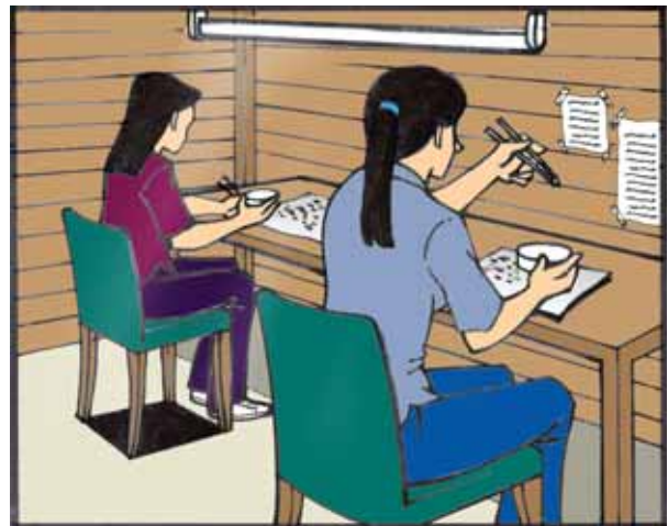
Figure 47: Provide bench lighting for work with small objects.
