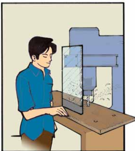
Figure 52: Transparent shield to prevent sawdust from reaching the worker.
