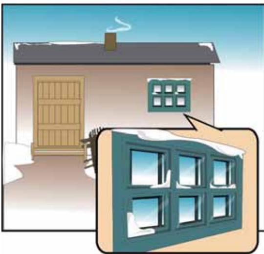
Figure 58: Double-layered window to prevent outside cold air from coming in.
