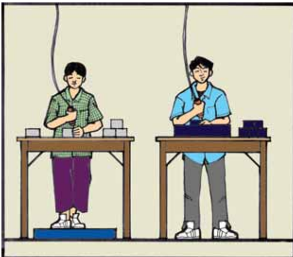
Figure 32: Use a foot platform for small workers and an item holder for tall workers to adjust their work height to their elbow levels.
