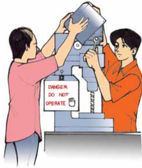
Figure 22: While maintaining or repairing a machine, the machine must be switched off and the electricity disconnected. Hang a tag, “DANGER, DO NOT OPERATE THE MACHINE”.
