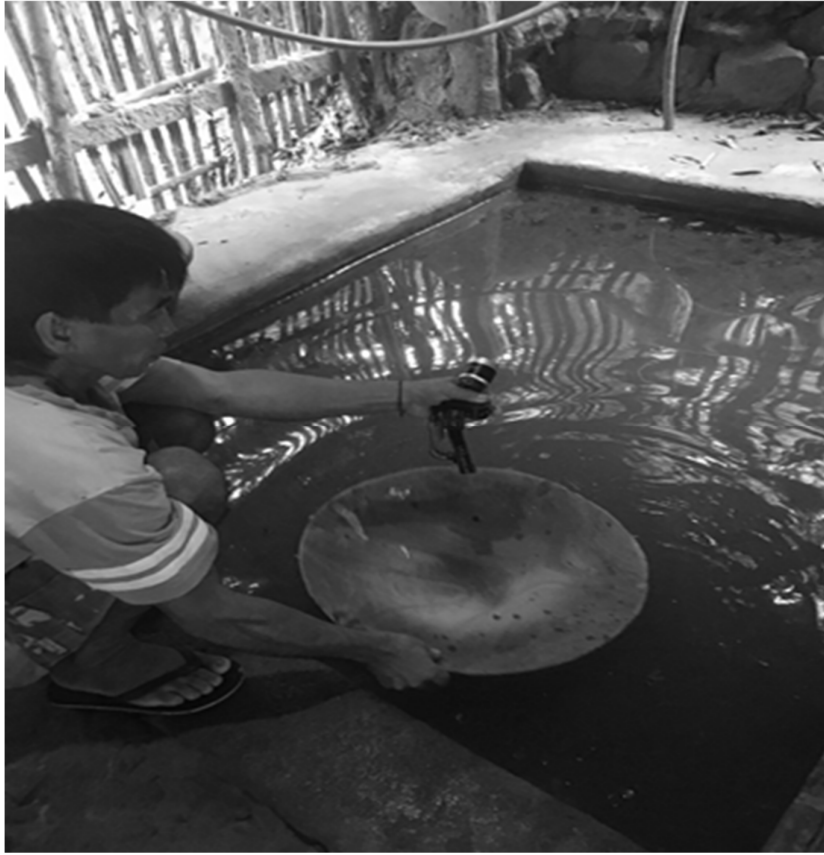
Figure 2. Mercury is being used to separate gold particles from rocks. The processing area is behind the house of the miner.
