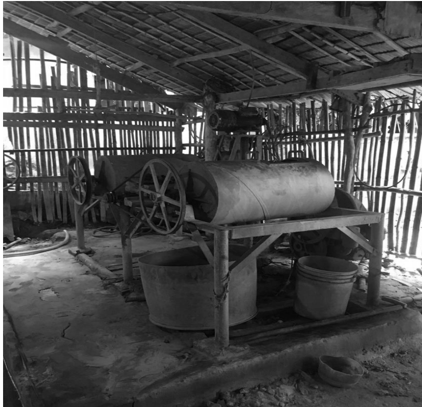
Figure 1. A ball mill machine used to mechanically break the ore. The machine is owned by a family that mines behind their house.
