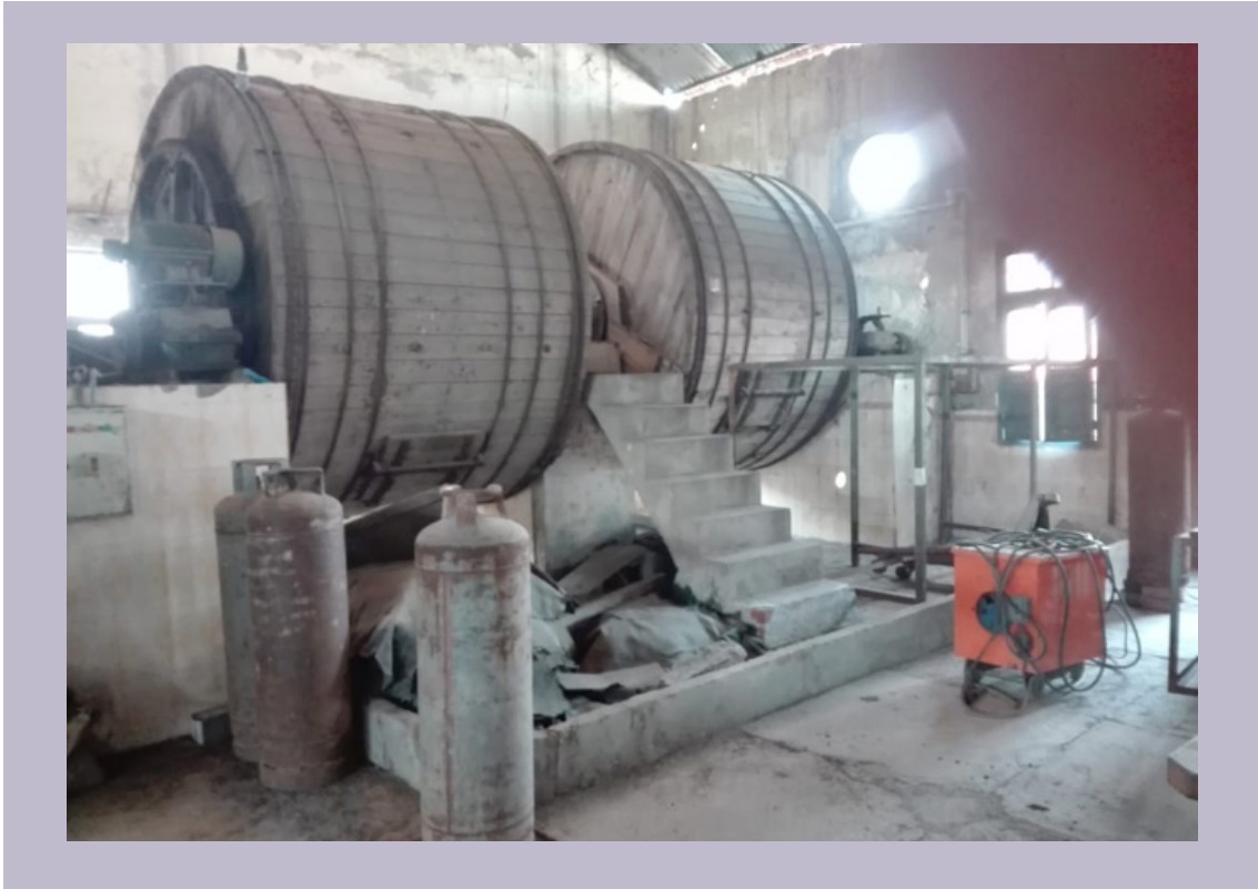
Figure 4. Tanning drums at the government-run Leather Service Centre, Kasur
