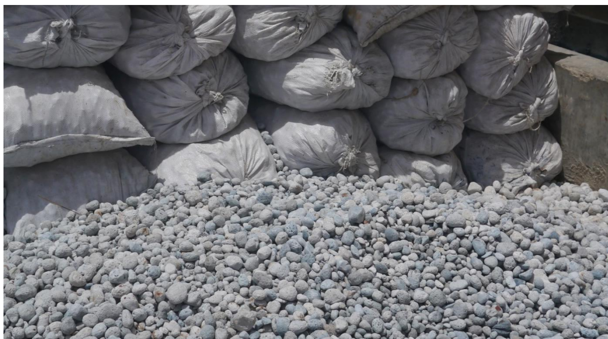
Stones used in the washing process in an export-oriented denim factory
